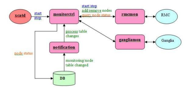
To use this infrastructure, first create a monitoring plug-in module and put it under /opt/xcat/lib/perl/xCAT\_monitoring/ directory. If the file name is xxx.pm then the module name will be xCAT\_monitoring::xxx.
