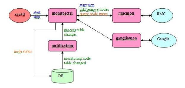
To use this infrastructure, first create a monitoring plug-in module and put it under /opt/xcat/lib/perl/xCAT\_monitoring/ directory. If the file name is xxx.pm then the
