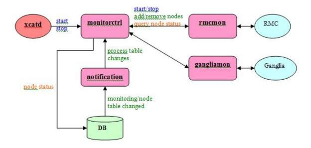
To use this infrastructure, first create a monitoring plug-in module and put it under /opt/xcat/lib/perl/xCAT\_monitoring/ directory. If the file name is xxx.pm then the package name will be xCAT\_monitoring::xxx. The following is a list of subroutines that a plug-in module must implement:
